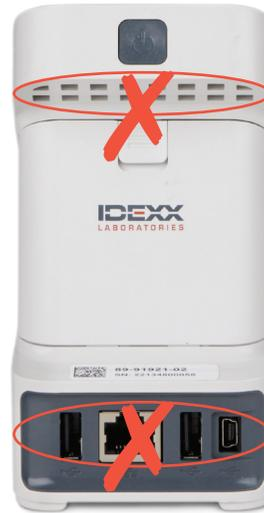
Clean the case and screen using a lint-free cloth dampened with 70% isopropyl alcohol, mild liquid soap and water, or a 10% bleach solution.
