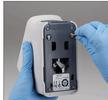
7. Turn the silver fasteners clockwise a quarter turn to lock the base into place.
