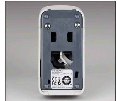
8. Ensure the base and silver fasteners are flush with the analyser and locked into place. **Not locking the base and fasteners properly can impact analyser performance.**
