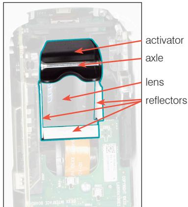
5. Clean the 3 white reflectors, the axle, and the activator using a new lint-free wipe or cotton swab dampened with 70% isopropyl alcohol, mild liquid soap and water, or a 10% bleach solution. **DO NOT clean the lens.**
