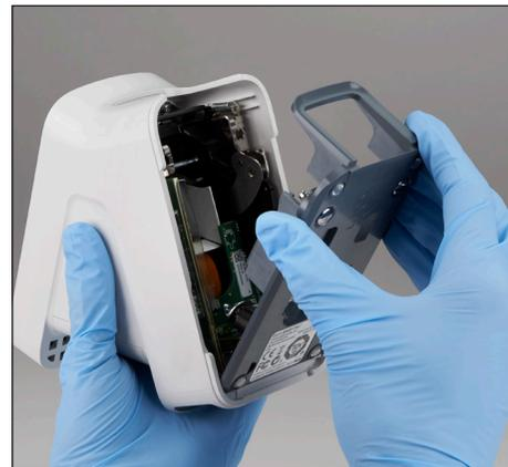
6. After the base has dried, reattach it to the analyser and ensure it is locked into place.
