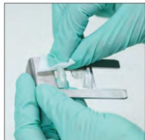
3. Remove the cartridge holder, clean it with a new alcohol prep pad, dry it with a new dry optical tissue, and then set it aside.
