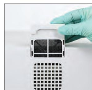
10. Remove the fan filter on the back of the analyzer, rinse it thoroughly with warm water, pat it dry with a paper towel, and return it to its location in the analyzer.
