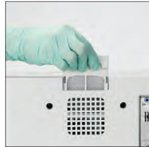
9. Return the waste bin, drip tray, centrifuge shield, and cartridge holder to their locations in the analyzer.
