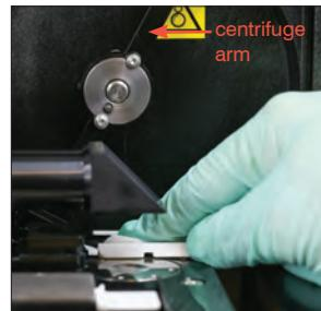
7. Gently move the centrifuge arm to the left and inspect the area below it for debris. If it's dirty, use a new alcohol prep pad to clean it and then dry it with a new optical tissue.
