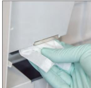
2. Open the analyzer door and clean the top and bottom of the pipetting window with a damp optical tissue. Then dry with a new dry optical tissue.
