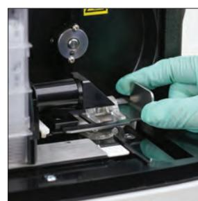
9. Return the waste bin, centrifuge shield, and cartridge holder to their locations in the analyzer.
