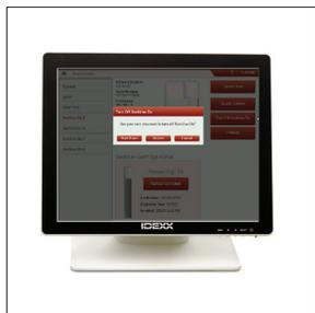
1. On the SediVue Dx Instruments screen, tap **Turn Off SediVue** and then tap **Shut Down**.
