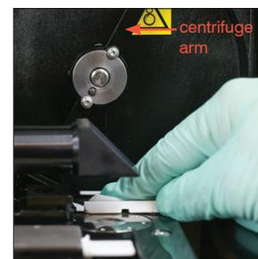
7. Gently move the centrifuge arm to the left and inspect the area below it for debris. If it's dirty, use a new alcohol prep pad to clean it and then dry it with a new optical tissue.
