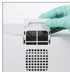
10. Remove the fan filter on the back of the Analyser, rinse it thoroughly with warm water, pat it dry with a paper towel, and return it to its location in the Analyser.
