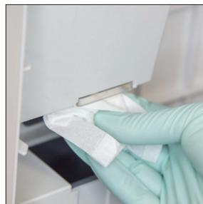
2. Open the Analyser door and clean the top and bottom of the pipetting window with a damp optical tissue. Then dry with a new dry optical tissue.
