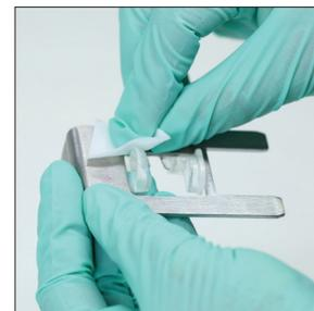
3. Remove the cartridge holder, clean it with a new alcohol prep pad, dry it with a new dry optical tissue, and then set it aside.
