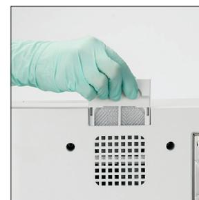
10. Remove the fan filter, rinse it thoroughly with warm water, pat it dry with a paper towel, and return it to its location in the Analyser. Then on the SediVue Dx Cleaning Guide screen, tap **Done** to power on the SediVue Dx.
