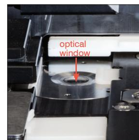
6b. Using a new alcohol prep pad (not rinsed), clean the optical window using a circular motion (3–4 times) and then dry it in a circular motion with a new dry optical tissue.
