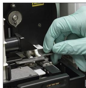
9. Return the waste bin, drip tray, centrifuge shield, and cartridge holder to their locations in the Analyser.
